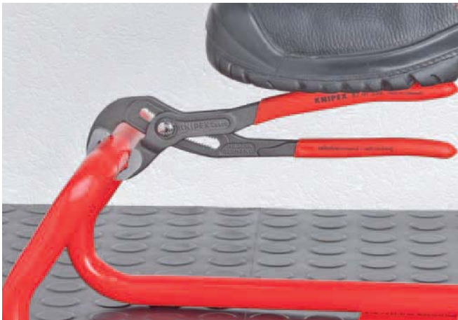
Teeth set against the direction of rotation have a self-locking effect and prevent slipping on the workpiece.
