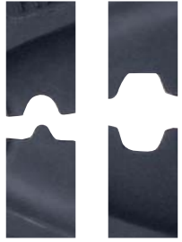
Crimping of the end caps on the Bowden cable sheath
