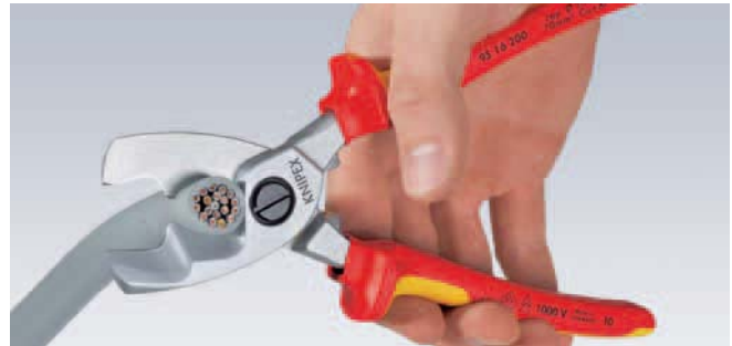
Final cut: after cutting the sheath in the front profile the cut is finished through the metal part of the cable in the rear profile. Initial cut in the front profile, final cut in the rear profile - to keep it as easy as possible.
