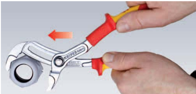
Quick setting without using a push-button
