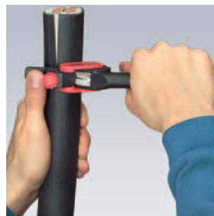
Turning the tool for circumferential cut
