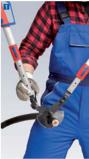
Setting of a favourable handle width
