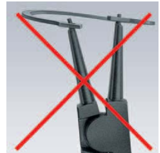
Conventional Circlip Pliers: distortion of the circlip when widening the circlip
